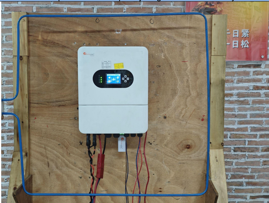
Set-up for Voltage Dips and Interruptions Immunity
