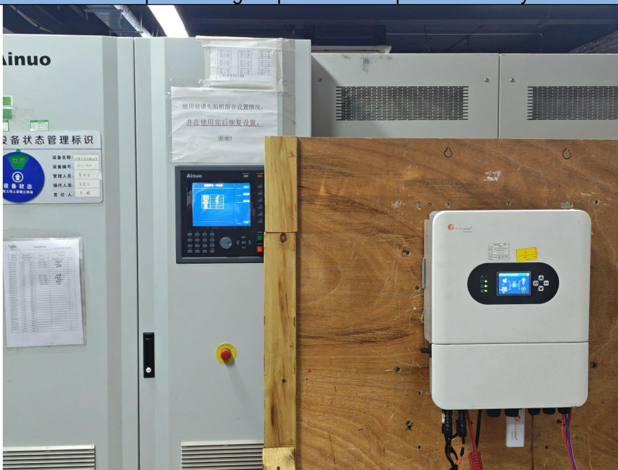
Set-up for Voltage Dips and Interruptions Immunity
