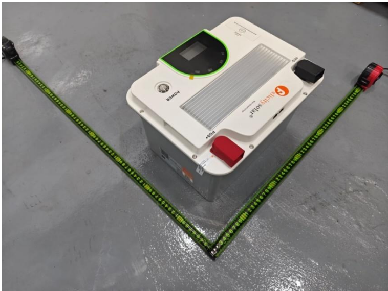
Battery: FLA12171-EU, 12.8V, 171Ah, 2.2kWh
