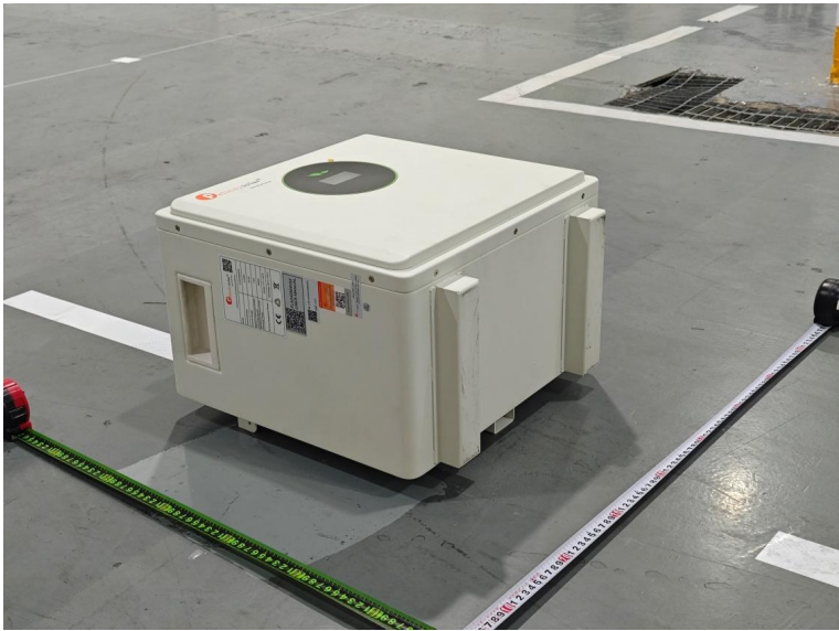
Battery: FLA24250WG2, 25.6V, 250Ah, 6.4kWh
