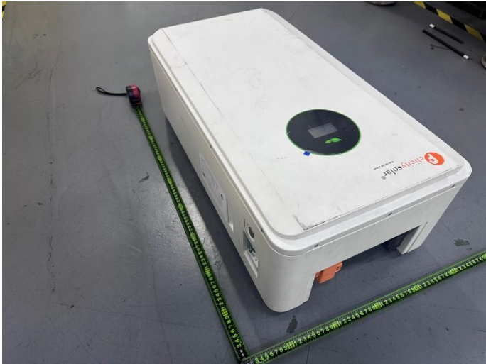
Battery: FLA24460-EU, 25.6V, 460Ah, 11.7kWh
