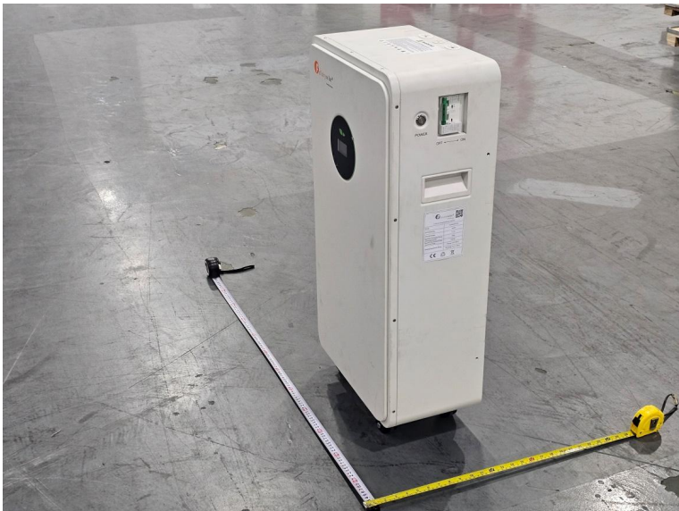
Battery: FLA48300TG2, 51.2V, 300Ah, 15kWh
