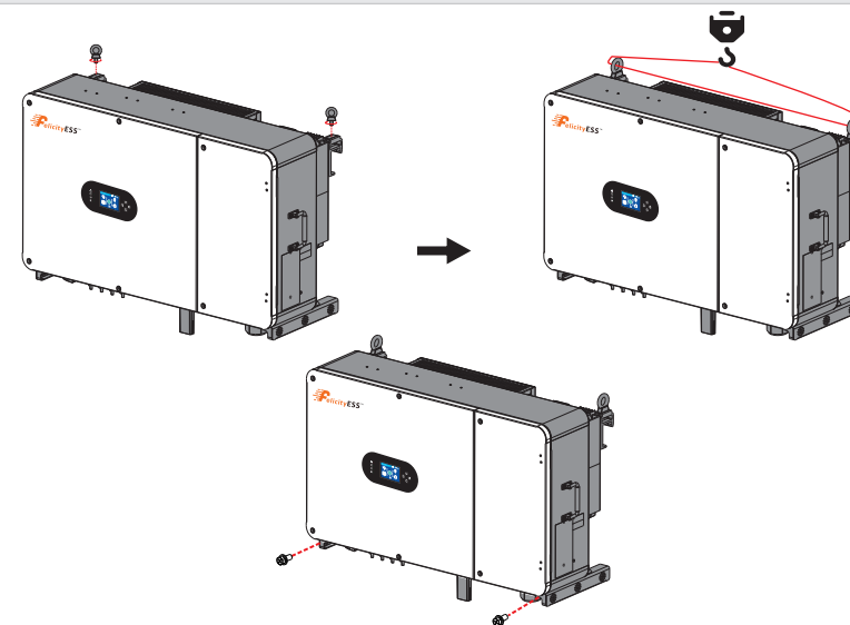
Figure 3.4-2 Installing an Inverter
